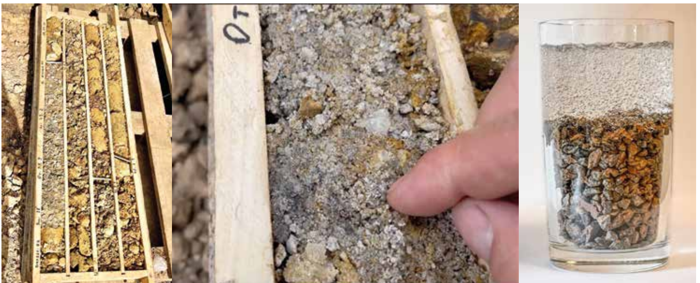
TORNADO + X-TEND 400: Stabilization of fractured rocks, 100% core recovery, prevention of drilling fluid loss.
